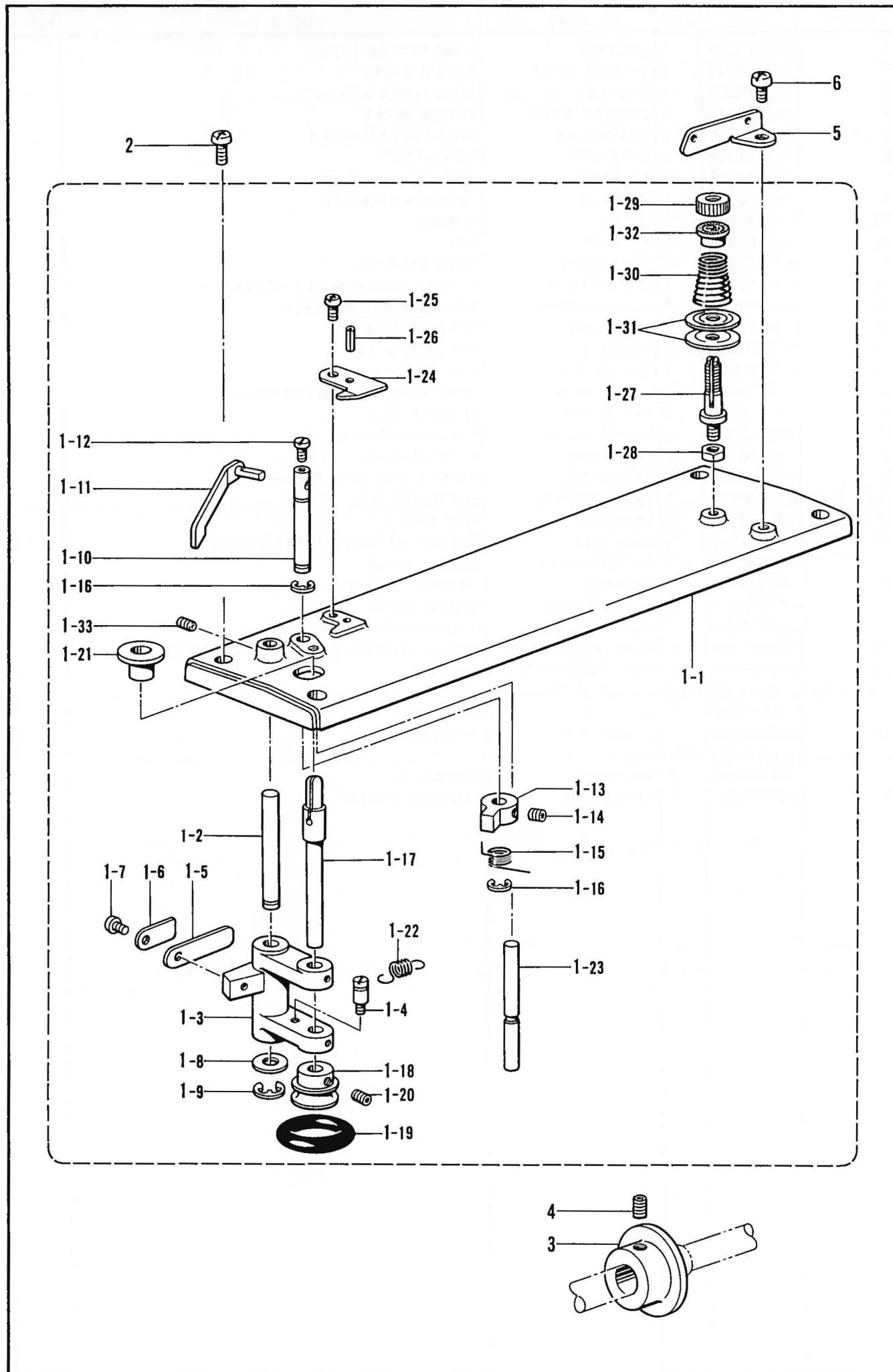
J. 糸巻関係 / Bobbin winder mechanism / Spuler /
