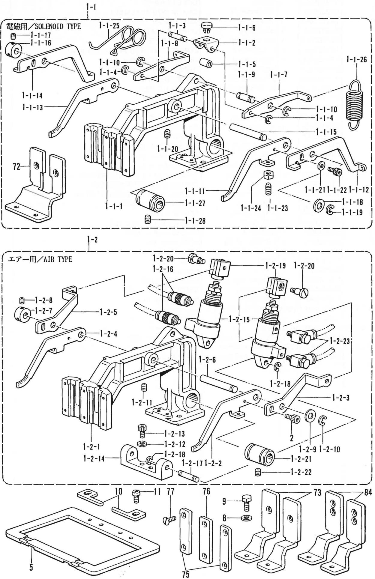
C1. 送り関係 / Feed mechanism / Transportvorrichtung /
